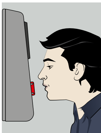
Passive test with an Alcolizer Centurion Zero Tolerance instrument
