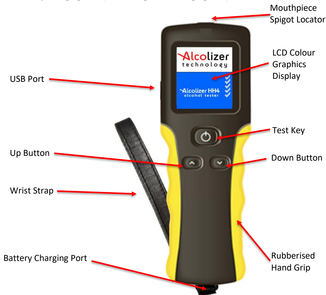
Figure 1 - User Display, Buttons and Adapter Sockets
