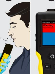
The device will analyse, emit a long beep, and then display a text based result.
