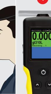
**A green screen** with "0.000g/210L" BrAC indicates that **alcohol** is not detected.
