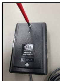
Unscrew the RFID card Reader
