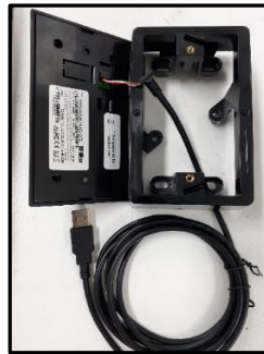
Removal of the RFID card Reader
