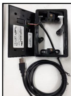
Removal of the RFID card Reader
