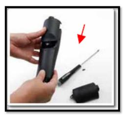
d. Do up the single screw on the back of the main module.
