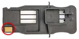
The electrical contact of the memory chip PCB can be affected by oxidisation or contamination, leading to poor electrical connectivity, and subsequent data transfer problems. The contacts can simply be wiped with a cloth damped with isopropyl or an eraser. **Do not** spray isopropyl or any other fluid near the cartridge, the strips must not be damaged.
