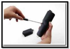
b. Slide off the out-of-calibration sample module.
